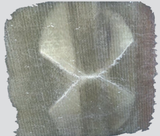
Figure 1: Image of H-Crack near CoG.
