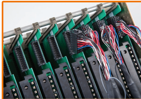
Connect cable with connector to adaptor card
