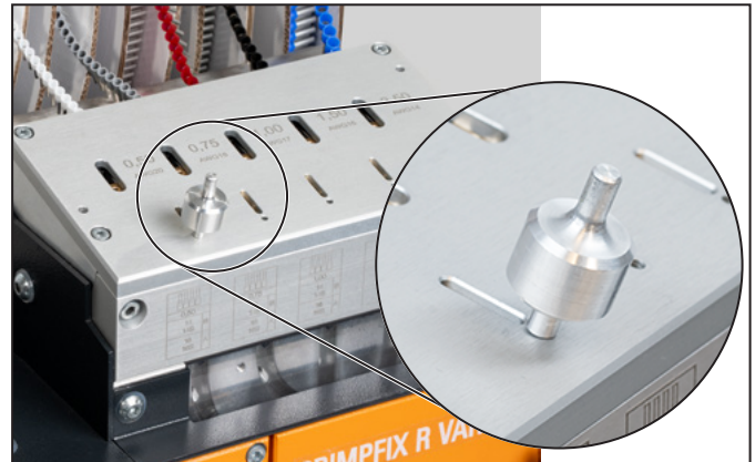
Figure 5.3 Fixing the wire-end ferrule belt
