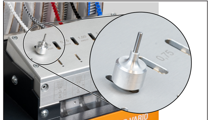
Figure 5.9 Releasing the wire-end ferrule belt
