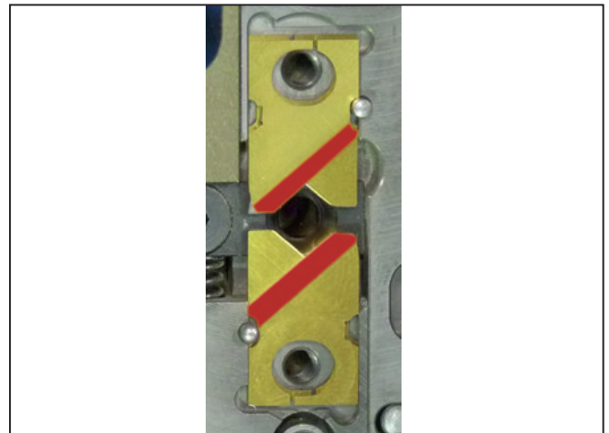
Figure 9.2 Insertion des lames
