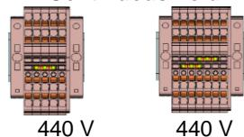
**C - Adjacent – separated by an end plate no difference between one or two cross-connections**
