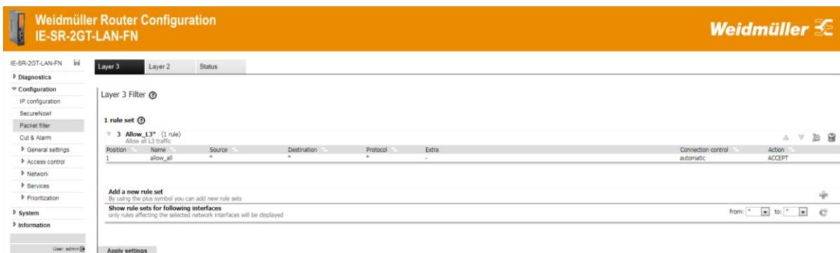
Figure 24: Factory default settings of Layer-3 Packet filter (firewall), valid for operation mode “IP Router”
