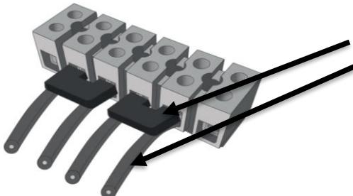
Assembly of the external cross connections QB 2 MK6:
