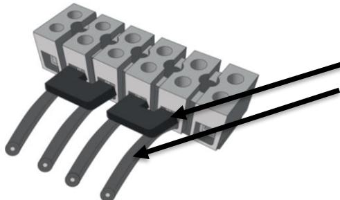
Assembly of the external cross connections QB 2 MK3 or QB 4MK 3:
