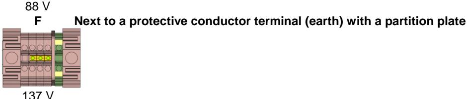
**F** Next to a protective conductor terminal (earth) with a partition plate
