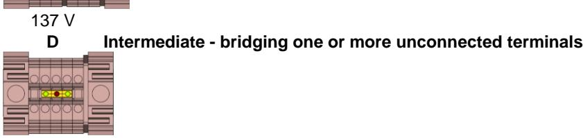
**D** Intermediate - bridging one or more unconnected terminals
