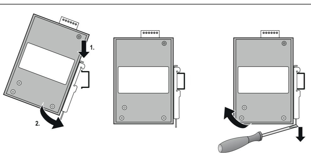
1. Place the mounting clip from above onto the DIN rail.
