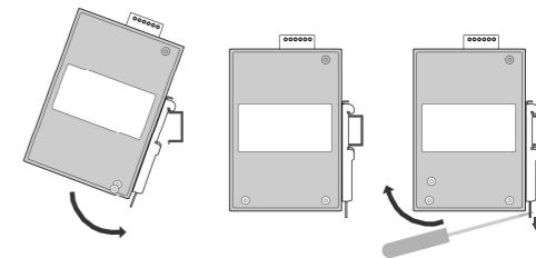
To remove the Ethernet Switch from the DIN-rail pull down the latch with a screwdriver then move the device away from the DIN rail and lift it up.
