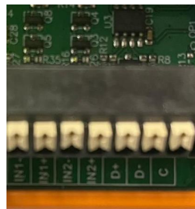
Image 2. RS-485 connectors from a Solar SMS
