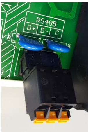
Image 1. RS-485 connectors from a Transclenic
