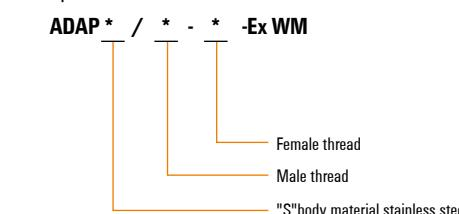
For example: ADAPS M20 -NPT 1/2- WM stainless steel adaptor, with male thread M20 thread to female thread NPT1/2.
