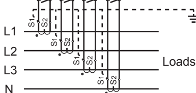
Fig.: Connection example, current measurement via current transformers
