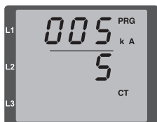
Fig.: Current transformer programming mode The primary and secondary currents can be changed using buttons 1 and 2 (cf. page 21).
