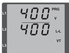
Fig.: Programming mode Voltage transformer The primary and secondary currents can be changed using buttons 1 and 2 (cf. page 21).
