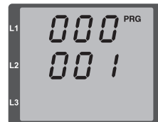
Fig.: Programming mode Parameter display The individual parameters can be changed using buttons 1 and 2 (cf. page 55).
