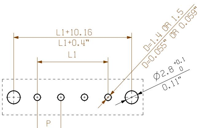
For the mounting of PCBs, it should be noted that the rated data given in the catalogue relates only to the connection elements. The necessary creepage and clearance paths must be observed in connection with the respective applicant in accordance to VDE 0110. The current-carrying capacity and pitch tolerance is to be determined according to IEC 60326 part 3 very fine.
