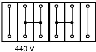
**D - Intermediate - bridging one or more unconnected terminals**
