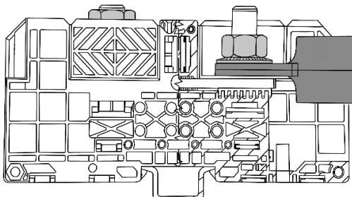
cable lugs of neighbouring terminals have to be installed parallel to each other.
