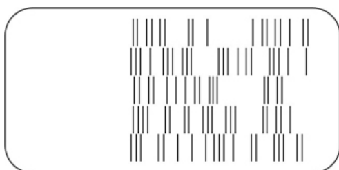
Figure 6.5 Print image: Approx. 50% functional nozzles
