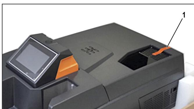
Figure 4.1 Transport restraint
