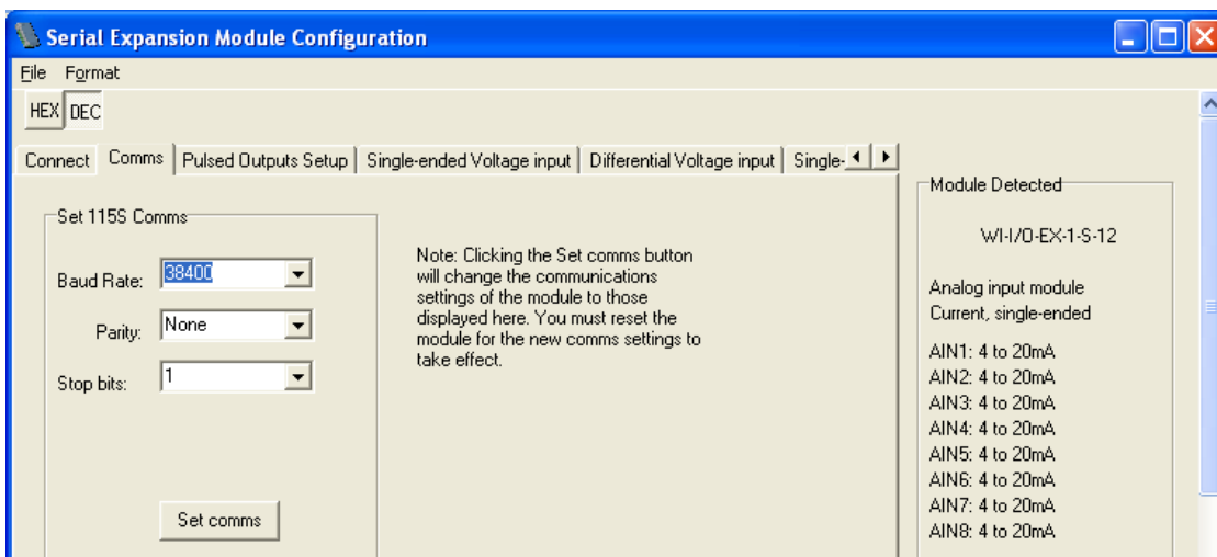
Figure 4-2: Communications configuration screen.
