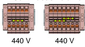
**C - Adjacent – separated by an end plate no difference between one or two cross-connections**
