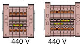
**C - Adjacent – separated by an end plate no difference between one or two cross-connections**
