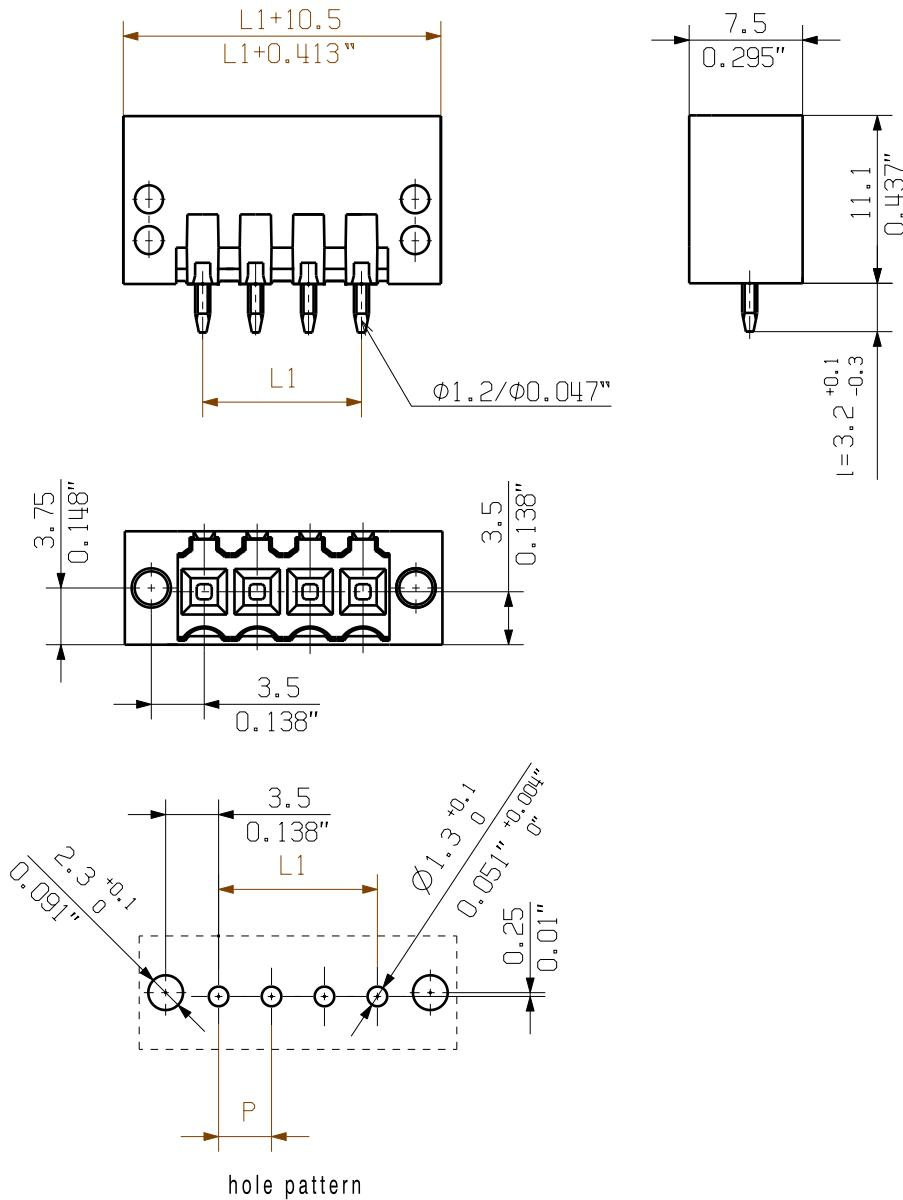
For the mounting of PCBs, it should be noted that the rated data given in the catalogue relates only to the connection elements. The necessary creepage and clearance paths must be observed in connection with the respective applicant in accordance to VDE 0110. The current-carrying capacity and pitch tolerance is to be determined according to DIN IEC 326 part 3 very fine.
