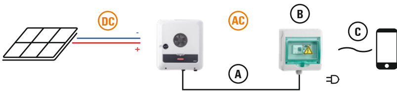
(A) 1 phase cable (B) Emergency power box (C) 1 phase cable with plug
