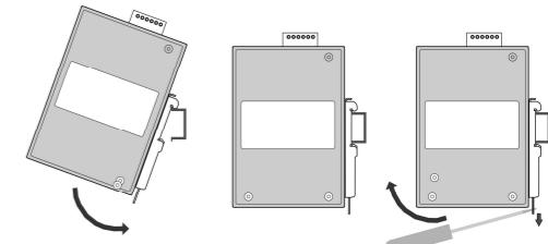
To remove the DIN-rail from the Ethernet Switch, simply reverse Steps 1 and 2.
