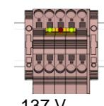
**F - Next to a protective conductor terminal (earth) with a end plate**
