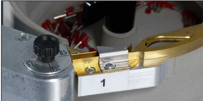
Figure 5.1 Ferrule cross section adjustment wheel (set: 0.5)
