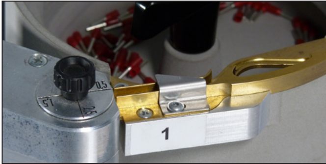
Figure 5.1 Ferrule cross section adjustment wheel (set: 0.5)
