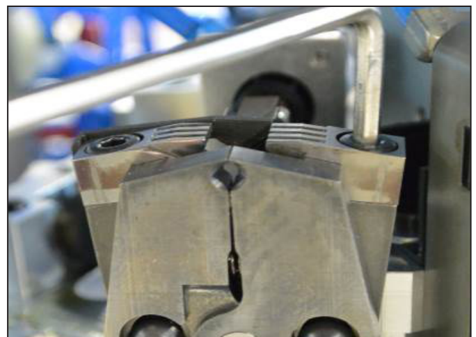
Figure 7.7 Removing PZ3 crimp dies
