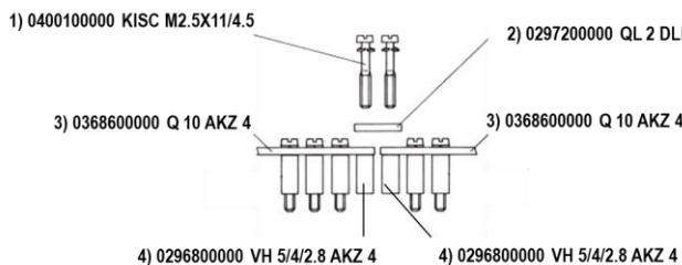
The AKZ 4 terminal include the option of setting up a cross-connection with more than 10 poles, e.g. 20-pole: 2 No. Q 10 (3) + 1 No. QL 2 (2). The end fixing screws are removed from the Q 10 (3) links by unscrewing them from the VH (4) sleeves. The QL 2 (2) is positioned between these and the two fixing screws (1) screwed into their VH sleeves again. This arrangement allows 20 poles to be cross connected.
