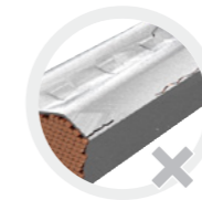
Cracks forming at the impressions of the crimping jaw
