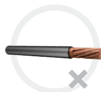
Damaged or cut-off individual strands
