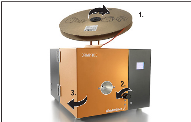
Figure 5.6 Positioning the wire-end ferrule
