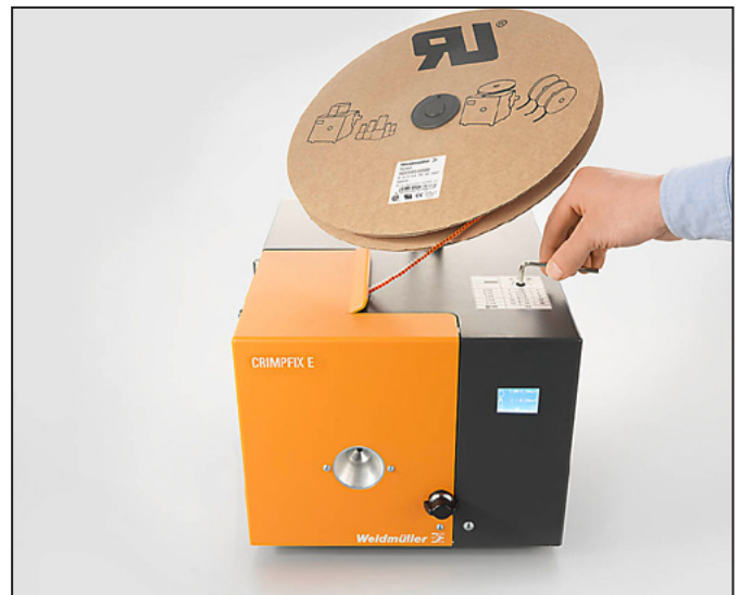
Figure 5.2 Stripping grade adjustment
