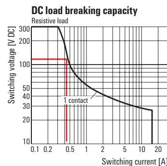
The curve shows a maximum switching current of approx. 0.45 A with resistive load. This must now be set in relation to the rated current of the relay (16 A) from the data sheet and the value for a DC13 load from the table.
