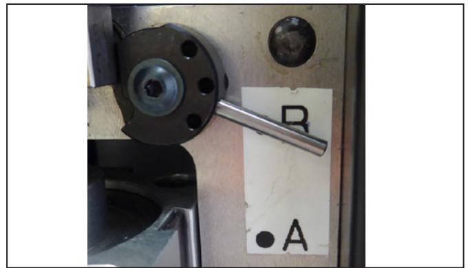
Figure 5.6 Stranded wire fixing unit configuration (set: B)
