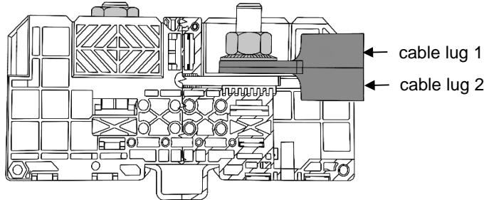
The cable lugs of neighbouring terminals have to be installed parallel to each other.
