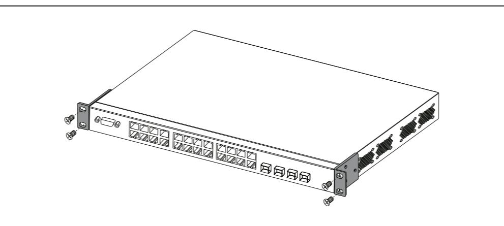
The Ethernet switch is delivered with the mounting brackets installed on the side of the data ports. With this arrangement, all data ports are located on the front panel when the Ethernet switch is installed in the 19" rack.
