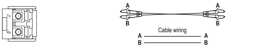
For a LC-Port with separate transmit and receive ports please remember to connect the Tx (transmit) port of device 1 to the Rx (receive) port of device 2, and the Rx (receive) port of device 1 to the Tx (transmit) port of device 2.
