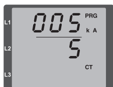
Fig.: Current transformer programming mode: Use button 1 and 2 to change primary and secondary current (see page 30).
