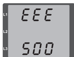
Fig.: Warning message with number 500 (mains frequency)
