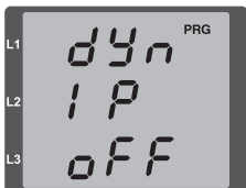
Fig.: Disabled dynamic allocation (dYn IP) of the TCP/IP address
