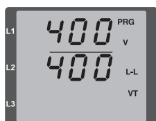
Fig.: Programming mode voltage transformer: Use button 1 and 2 to change primary and secondary voltage (see page 30).
