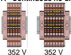
**C - Adjacent – separated by an end plate no difference between one or two cross-connections**
