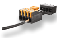
MPS / MHS 5 20 - 12 AWG (0.5mm 2 - 4.0mm 2 ) 300V / 18.5A UL 2 - 12 poles
