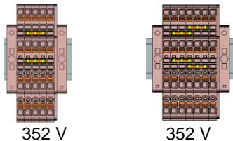
**C - Adjacent – separated by an end plate no difference between one or two cross-connections**
