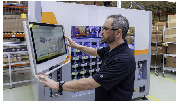
Automated DIN-Rail assemblers can drastically reduce manual build time and expense for terminal rail assembly and wire preparation.
