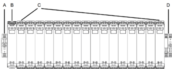
Figure 9: Arrangement of the components A End bracket WEW 35/1, mechanical B ACT20C gateway C ACT20C modules (1...16) D ACT20C bus termination terminal
