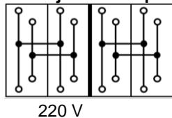
**D - Intermediate - bridging**
