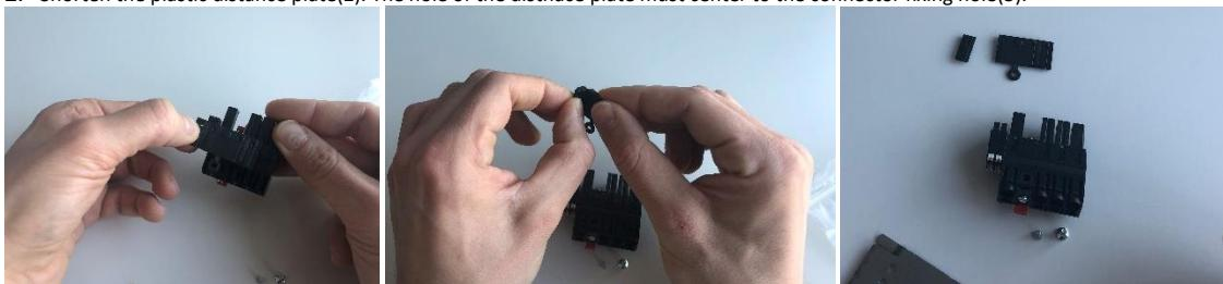
3. Fix the distance plate(2) to the connector by the dovetails and center the hole of the distance plate to the connector fixing hole(3).
