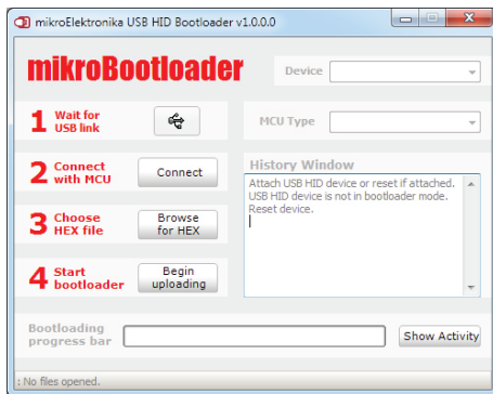
Figure 3: Bootloader PC application software used to upload instrument firmware updates.
