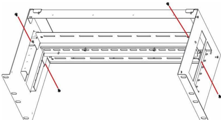
**Step 4:** Attach RM-KIT into a 19"-rack cabinet and then mount the device onto RM-KIT.
