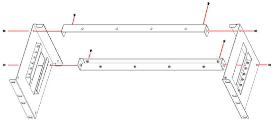
**Step 2:** Fix din rail one to the panel.
