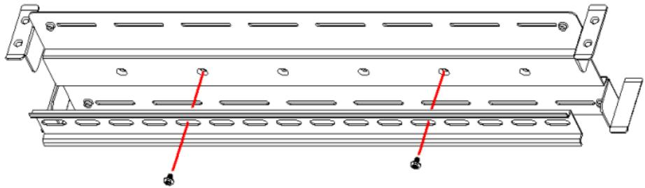
**Step 3:** Determine the depth by adjusting the position of panel and then fix it with 4 screws.
