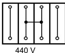
**C - Adjacent – separated by an end plate**
